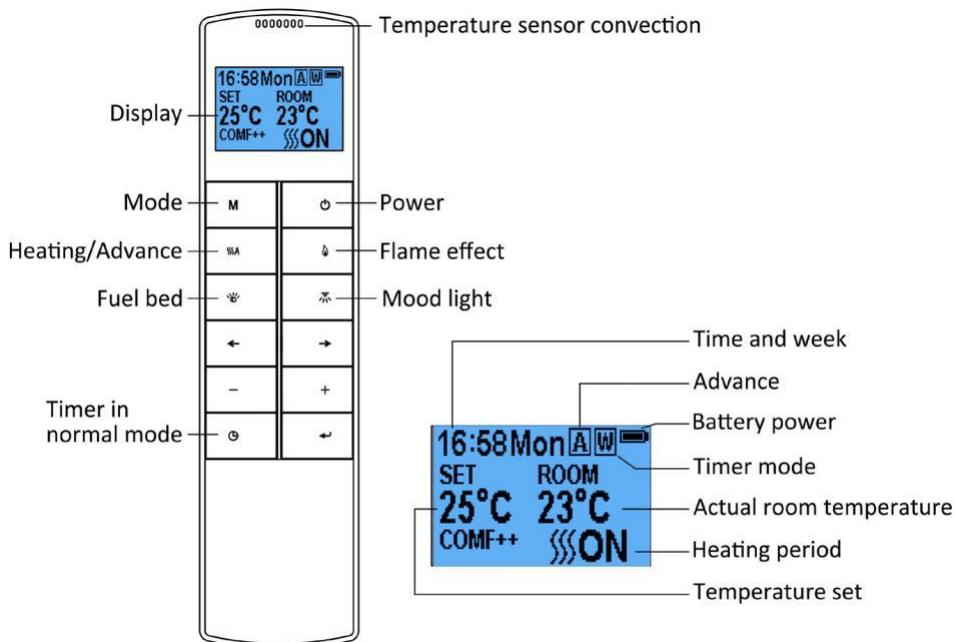
**NOTE: This is a thermostatic remote control. The remote should be in the same room as the fireplace and placed on a flat surface. It must be placed away from the fire so the hot air will not blow on it and affect the thermostatic reading.**
