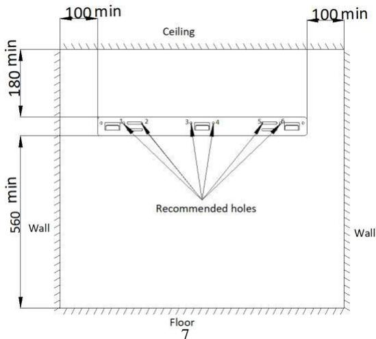
5.3c Tap the plastic wall plug into the six holes. Then use five ST5\*40 screws to fix the brackets on the wall.
